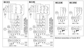
Electrical connections of heater BC
